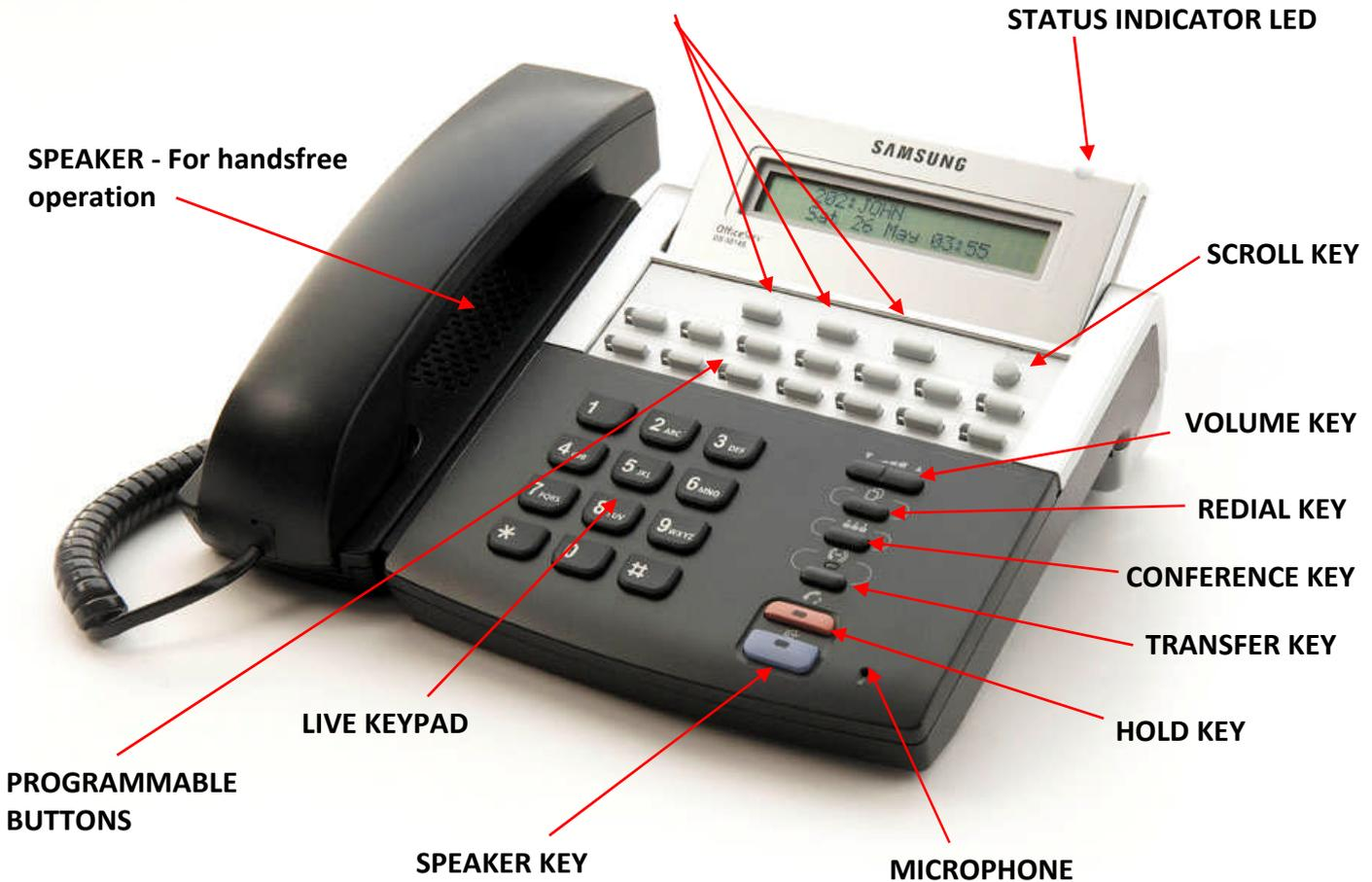
The **programmable buttons** above the keypad are arranged in rows of 1x7 (7) buttons, or 2x7, (14) buttons or 3 x7 (21) buttons and are numbered from 1 to 7 or 14 or 21 from top left to bottom right. By default, keys 1 and 2 are set as Call keys. Call keys flash for incoming calls.
